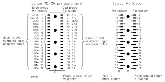
**Pin 1 and pin 3** These pins are +5 volt and DC return for +5 volt supply. You can use 800 ma per probe up to a total of 10 amps for 20 probes. The logic analyzer supplies the power.
